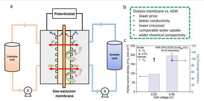
Fig. 6 Bipolar H<sub>2</sub> production in the system with a dialysis membrane. (a) Scheme of the flow cell with a dialysis membrane. (b) Comparison between the dialysis membrane and AEM. (c) Partial current densities of H2 at different cell voltages with 250 ml of electrolyte.
