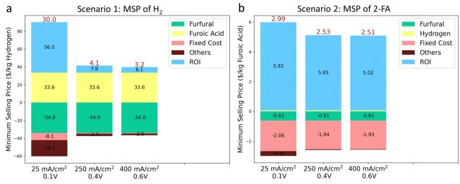
Fig. 7 Techno-economic analysis (TEA) for the bipolar  $H_2$  production system. (a) Minimum selling price (MSP) of  $H_2$  and (b) 2-FA at three different current densities and cell voltages. The electrochemical plant capacity is 1500 kg/day of  $H_2$ .
