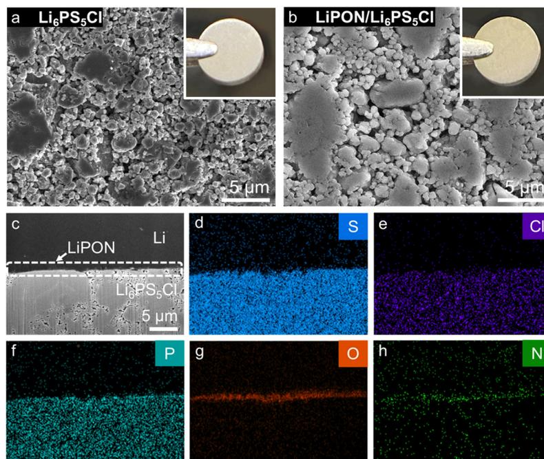
Fig. 2 Top-view SEM images of the surface morphologies of the Li<sub>6</sub>PS<sub>5</sub>Cl pellet (a) without and (b) with LiPON coating. The upper-right insets are digital photos of the bare Li<sub>6</sub>PS<sub>5</sub>Cl and LiPON coated Li<sub>6</sub>PS<sub>5</sub>Cl pellets. (c) FIB-SEM cross-sectional image of the LiPON coated Li<sub>6</sub>PS<sub>5</sub>Cl SSE and Li metal interface, with (d–h) corresponding EDX mapping images for S, Cl, P, O, and N.
