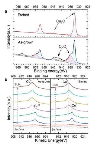
Fig. 5 (a) The surface XPS Cu 2p region of as-grown and etched TO-Cu<sub>2</sub>O. (b) Depth profile XPS of the Cu LMM Auger peak of as-grown and etched TO-Cu<sub>2</sub>O with a 5 nm ALD Ga<sub>2</sub>O<sub>3</sub> layer.
