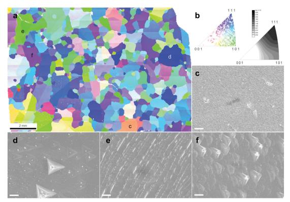
Fig. 3 (a) The orientation map shown with the inverse pole figure (IPF) colour key with respect to the surface normal direction of an etched TO-Cu<sub>2</sub>O. (b) The coloured figure is the legend of orientation and the grey figure with the scale bar shows the orientation density in the inverse pole figure with respect to the surface normal direction. (c-f) SEM images of corresponding sites in (a) with typical crystal orientations. The scale bar in (c-f) is 10 micrometres.
