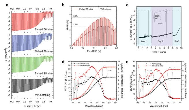
simulated AM 1.5 G irradiation (100 mW cm<sup>-2</sup>) in pH 7 electrolyte. (b) The comparison of ABPE of the unetched and etched (60 min) champion photocathodes. (c) The stability test of an etched sample (60 min) at 0.56  $V_{RHE}$  under simulated AM 1.5 G irradiation (100 mW cm<sup>-2</sup>) in pH 7 electrolyte. The IPCE and integrated photocurrent density of the unetched and etched (60 min) at (d) 0 V<sub>RHE</sub> and (e) 0.5 V<sub>RHE</sub>
