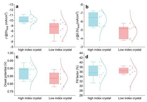
Fig. 4 Statistical PEC performance of high index (HIG) and low index (LIG) single crystal photocathodes. Photocurrent at (a) 0 V<sub>RHF</sub> and (b) 0.5 V<sub>RHF</sub>. (c) Onset potential. (d) Fill factor.
