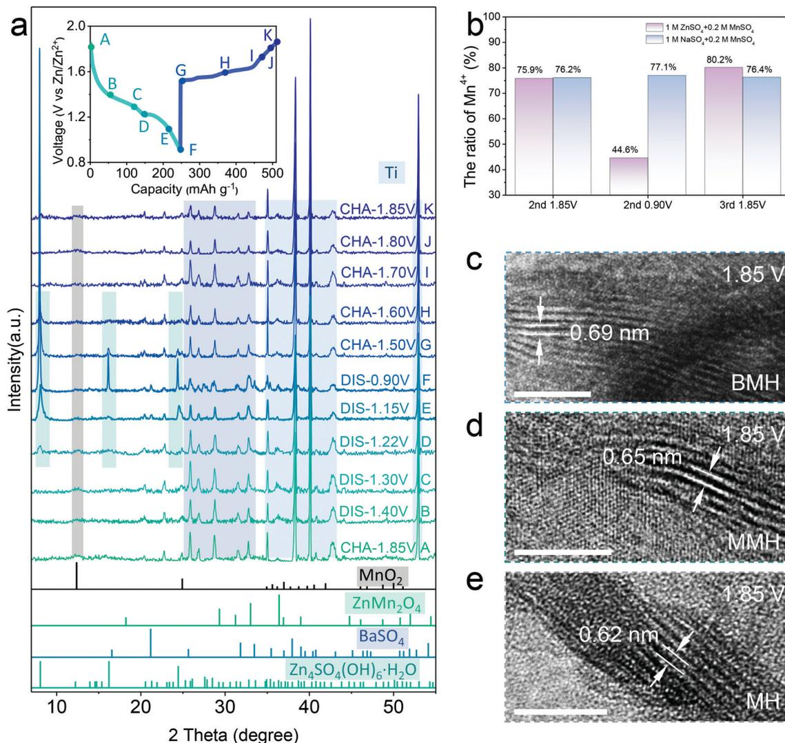
Fig. 2 Charge storage mechanism. (a) *Ex situ* XRD patterns of the BMH cathode in selected states in the 2nd discharge/charge cycle. (b) Analysis of reversible change in the ratio of  $\text{Mn}^{4+}$  at different states by XPS spectra in different electrolytes. (c–e) TEM images of three samples at the fully charged state of 1.85 V. Scale bar, 5 nm.
