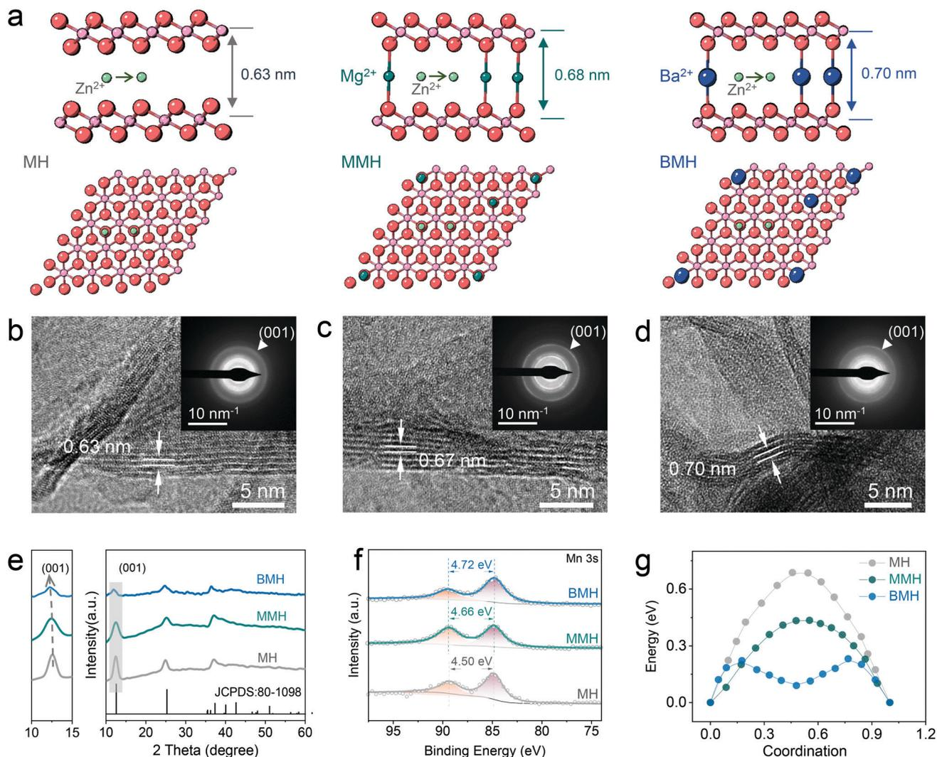
**Fig. 1** Design and characterization of MH, MMH, and BMH. (a) Calculation model and possible migration path of  $\text{Zn}^{2+}$ . (b–d) TEM images, (e) XRD patterns, and (f) XPS spectra of Mn 2p. (g)  $\text{Zn}^{2+}$  migration energy in different materials.
