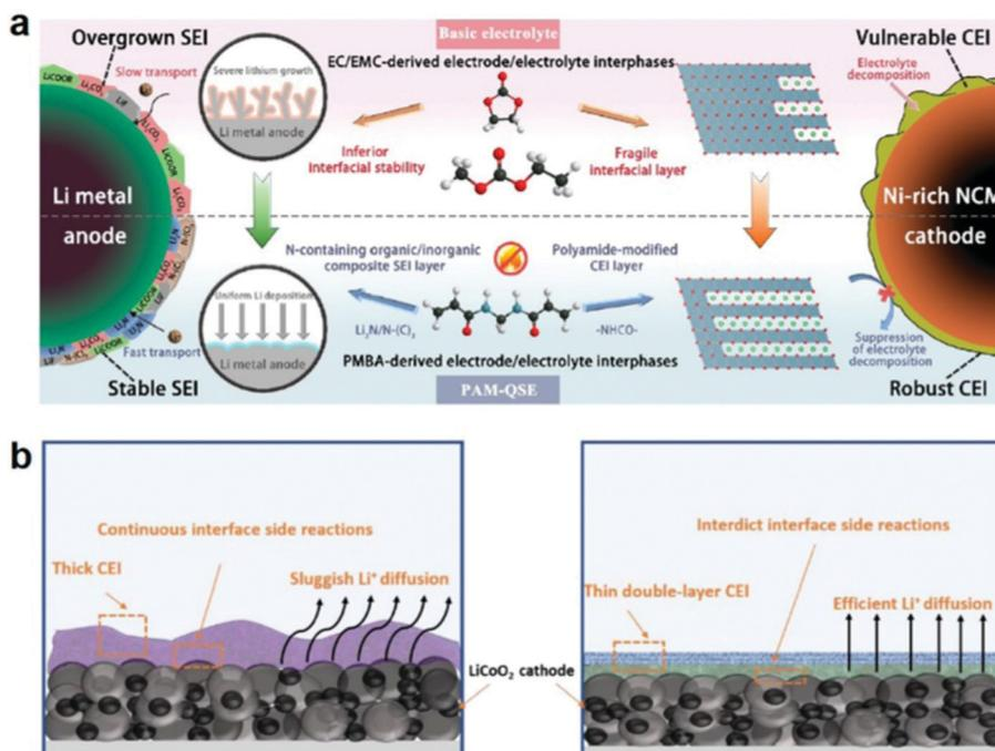
Fig. 5 (a) Design strategy for PAM-QSE: schematic illustration of the interface stabilization mechanism for PAM-QSE. Reproduced with permission.<sup>109</sup> Copyright 2020, Elsevier. (b) The thick CEI and the thin double-layer CEI formed in CPEs. Reproduced with permission.<sup>110</sup> Copyright 2021, Elsevier.
