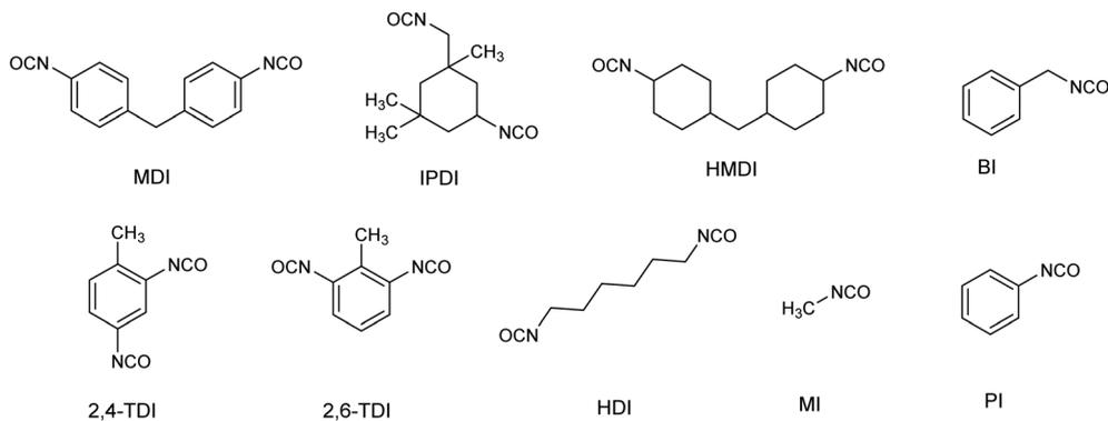
Fig. 1 Chemical structures of commercially important organic isocyanates.
