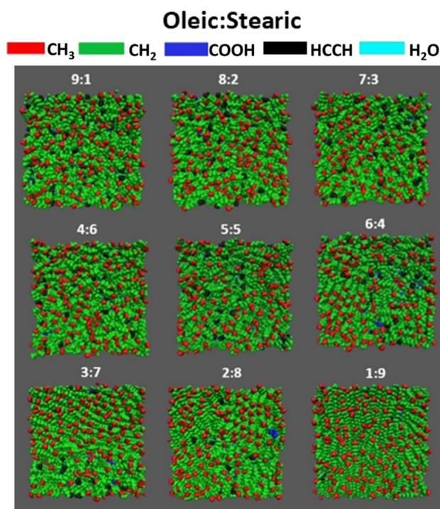
Fig. 4 Top-down views of the same slabs as shown in Fig. 3, with atoms highlighted based on functional group. Methyl groups are shown in red,  $\text{COOH}$  groups in dark blue,  $\text{CH}_2$  in green,  $\text{HC}=\text{CH}$  in black and water in cyan. Images have been made at the end of a 10 ns production run.
