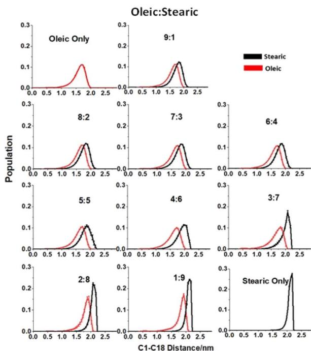
Fig. 6 Distributions of C1–C18 distances for different oleic:stearic ratios. Plots are averages over the top and bottom of four slabs, and at times >4 ns into a 10 ns production run. Error bars give one standard error of the mean and their small size indicates the consistency of these results. Distances have been binned into 0.05 nm bins.
