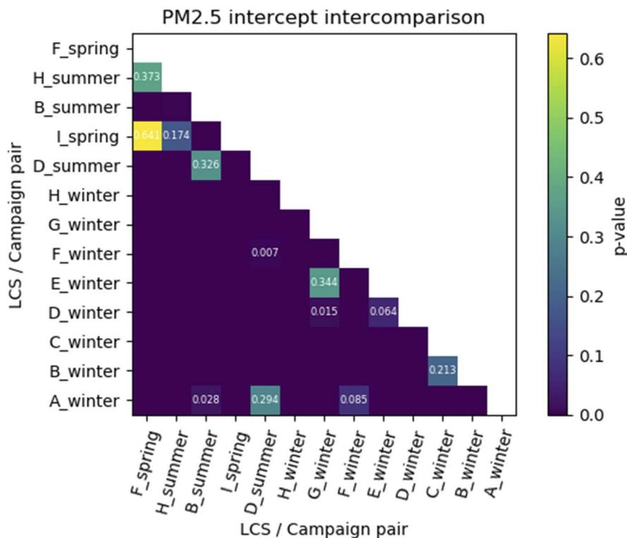
Fig. 5 Results of the *t*-test on the intercept pair for the PM<sub>2.5</sub> calibration. Only the *p*-values which indicate a null difference in means (*p*-value > 0.05, with a subsequent Bonferroni correction) are written on the plot.
