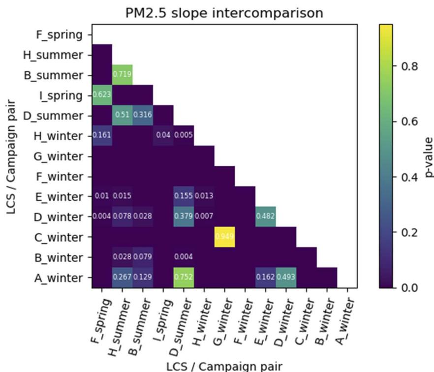
Fig. 4 Results of the statistical t-tests for the PM<sub>2.5</sub> data. Only the *p*-values which indicate a null difference in means (*p*-value > 0.05, with a subsequent Bonferroni correction) are written on the plot.
