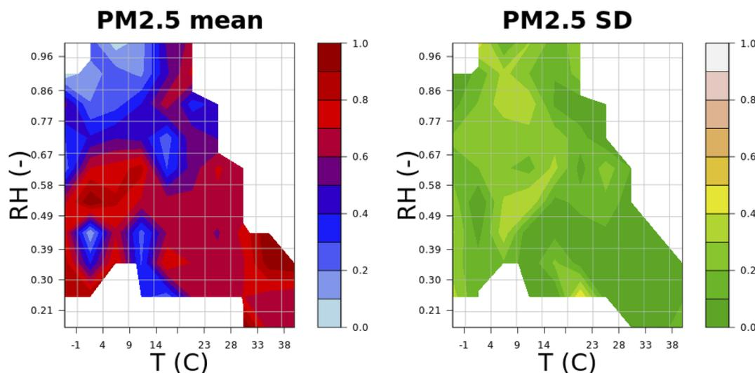
Fig. 8 Visualization of the BLUM-i. Fraction of the PurpleAir  $PM_{2.5}$  measurements meeting the criteria to be considered indicative (5 minute time resolution) as a function of temperature and relative humidity. Left panel: average and right panel: standard deviation.
