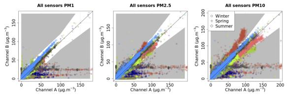
Fig. 1 Inter-channel performance of the PurpleAir systems for  $PM_1$ ,  $PM_{2.5}$  and  $PM_{10}$  (1 minute readings). Each color represents an individual system/campaign pair. The shaded areas represent measurements that do not meet the QA/QC criteria.
