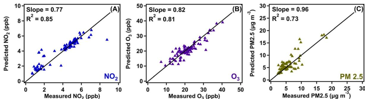
Fig. 3 Hourly averaged regression plots of pollutant data comparing the observed dataset with the predicted dataset output by the RF model for the during October 07–18, 2021 period for (A) NO<sub>2</sub>, (B) O<sub>3</sub>, and (C) PM<sub>2.5</sub>. Data collected from the Pod 2 location. The diagonal is the 1 : 1 line. The slope and  $R^2$  values are calculated from the regression of predicted onto observed.
