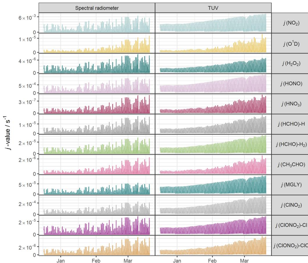
Fig. 2 Time series of hourly mean  $j$ -values for 12 photolysis reactions at Chilbolton Observatory from 17 December 2020 to 19 March 2021: left, as measured by spectral radiometer; right, as simulated by the TUV v5.3 model.
