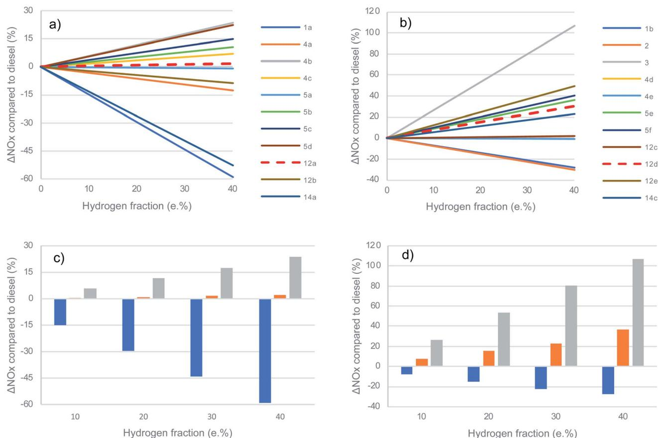
**Fig. 1** Meta-analysis of effect on NO<sub>x</sub> emissions for H2D combustion in large diesel engines for different H2D fuel compositions. (a) 0–30% low load case (b) 50–100% high load case. Numbers in the legend correspond to datasets in Table 1. The median dataset is presented as a red dashed line. (c) Worst (grey), median (orange) and best-case (blue) NO<sub>x</sub> scenarios for 0–30% load (d) worst (grey), mean (orange) and best-case (blue) scenarios for 50–100% load.
