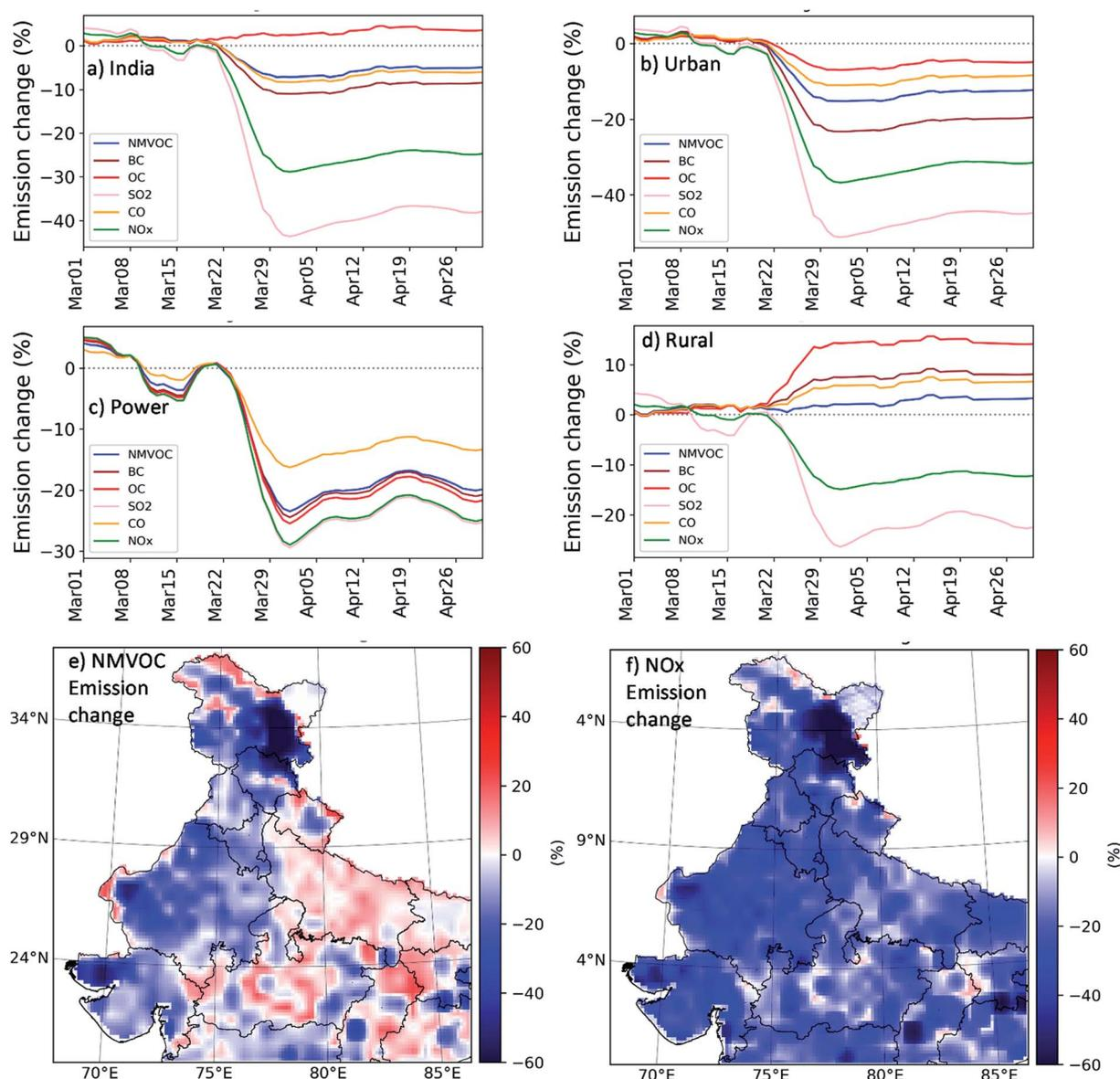
Fig. 2 Daily emission change due to AF applied on CEDS\_M emissions averaged in (a) India, (b) Urban, (c) Power, and (d) Rural (X-axis shows the days in March and April and the Y-axis range is different for each subplot). Map of emission changes of (e) NMVOC and (f) NO<sub>x</sub> averaged in April 2020. The location of the box regions can be found in the ESI.†
