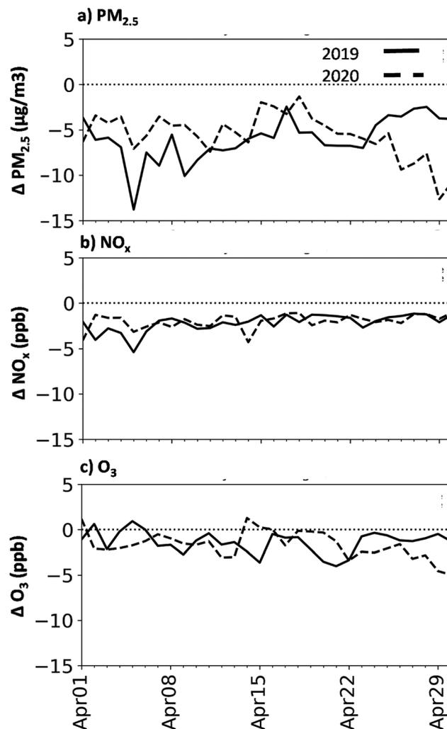
Fig. 6 Effect of lockdown emissions on daytime (a) PM<sub>2.5</sub>, (b) NO<sub>x</sub>, and (c) ozone concentrations in April 2019 (solid line; difference between 2019COVID and 2019BAU) and 2020 (dashed line; difference between 2020COVID and 2020BAU).
