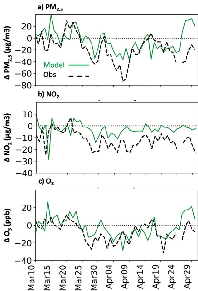
Fig. 4 Averaged daytime (1000–1700 LT) PM<sub>2.5</sub> (top row), NO<sub>2</sub> (middle row), and ozone (bottom row) concentration changes in 2020 and 2019, between 10 March and 30 April, based on the measured data over CPCB stations in Delhi (black dashed line) and modeled data (green solid line) over the Urban region. The observed data were extracted from the ground measurement data in Delhi, while the modeled data were averaged in the Urban box region.
