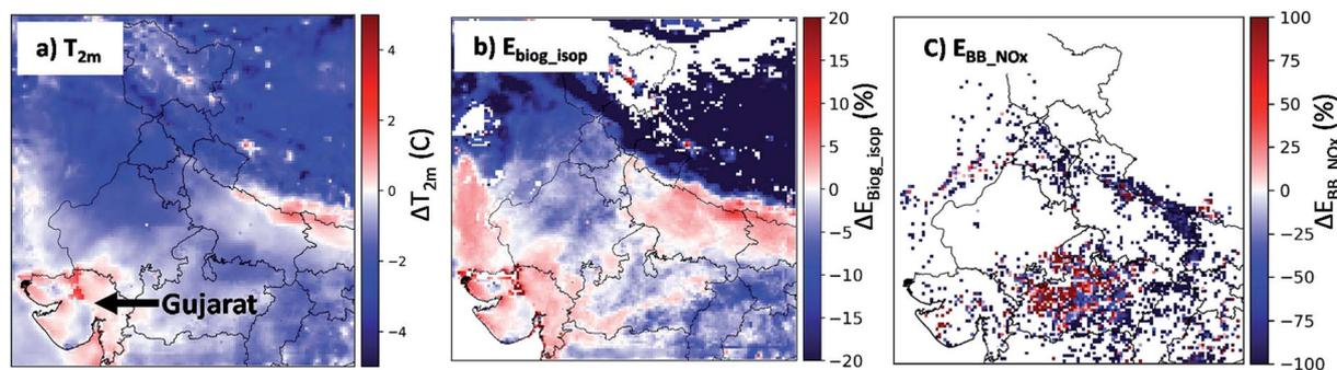
Fig. 5 Difference between April 2020 and 2019 in modeled daytime averaged (a) 2 m temperature, (b) biogenic isoprene, and (c) biomass burning NO<sub>x</sub> emissions over the domain. The changes in  $E_{BB\_NOx}$  are also true for other biomass burning species such as CO.
