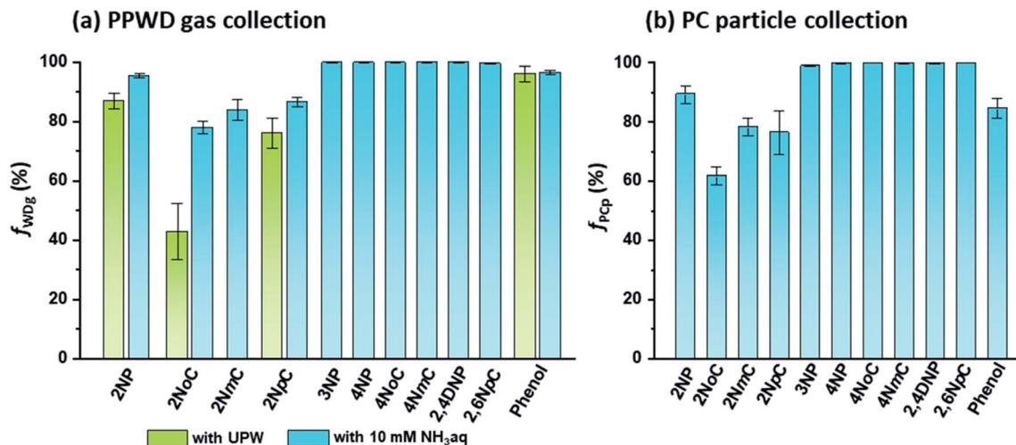
Fig. 5 Collection efficiencies of NPs and phenol for (a) gas collection by the PPWD ( $f_{WDg}$ ) and (b) particle collection by the PC ( $f_{PCp}$ ).
