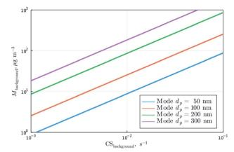
Fig. 8 Mass concentration of background aerosols as a function of their corresponding CS and mode diameter. The other model inputs are:  $\sigma_{\text{geo}} = 1.7 \text{ and } \rho = 1400 \text{ kg m}^{-3}$ .
