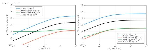
Fig. 5 Number, surface area and mass concentration of the growing mode after 48 h as function of the formation rate of 5 nm particles,  $J_5$ . The condensation sink of the background particle population,  $CS_{background}$ , has been assumed to be equal to  $0.010 \, s^{-1}$  (left panel) or  $0.001 \, s^{-1}$  (right panel). The other model inputs are: initial particle diameter = 5 nm, duration of NPF = 5 h,  $GR = 4 \, \text{nm h}^{-1}$  and  $\sigma_{GPO} = 1.7$ .
