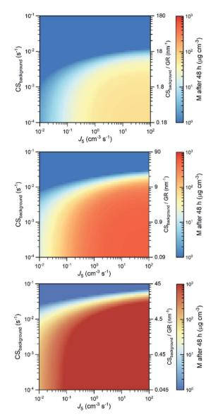
Fig. 7 Mass of the growing mode after 48 h as function of  $J_5$  and CS<sub>background</sub>. The other model inputs are: initial  $d_{\rm p}=5$  nm, duration of NPF = 5 h,  $\sigma_{\rm geo}=1.7$ , and GR is equal to 2 nm h<sup>-1</sup> (upper panel), 4 nm  $h^{-1}$  (middle panel) or 8 nm  $h^{-1}$  (bottom panel).
