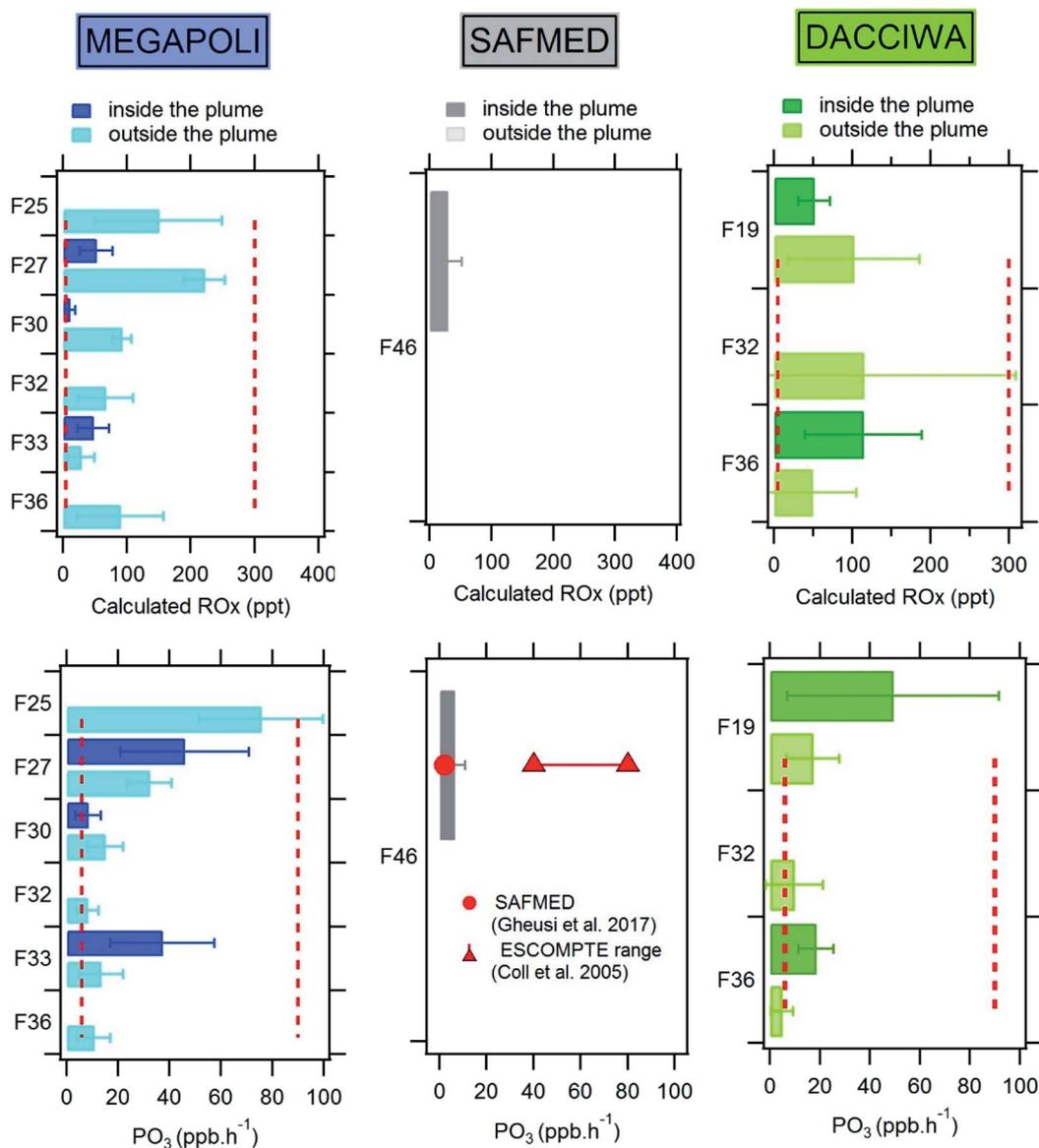
Fig. 10 Mean and standard deviations values of  $[RO_x]$  and ozone production ( $PO_3$ ) calculated from the PSS in Paris, WMB and SWA. Dashed lines (for MEGAPOLI and DACCIWA) are the range of values reported in the literature in the same region (see text for references).
