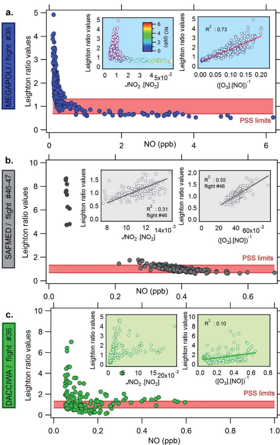
Fig. 9 Scatterplots of  $\Phi$  versus NO mixing ratios during the three campaigns: flight 36 for MEGAPOLI, combined flights 46 and 47 for SAFMED and flight 36 for DACCIWA. Scatterplots are color-coded with  $J(\text{NO}_2)$ . The background-colored scatterplots represent the correlation of  $\Phi$  with the PSS terms.
