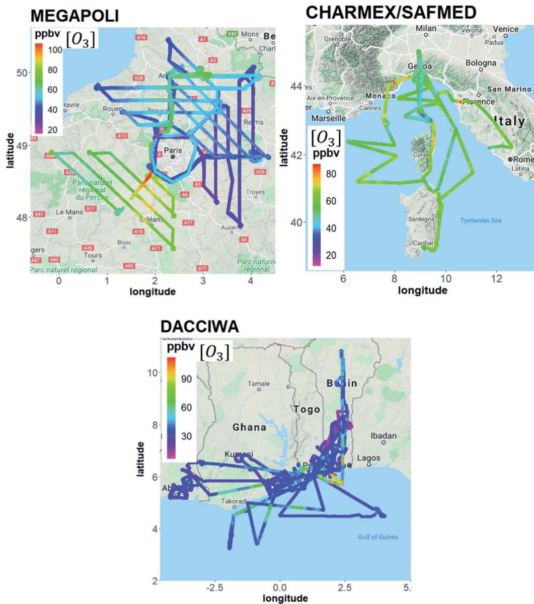
Fig. 2 MEGAPOLI, ChArMEX/SAFMED and DACCIIWA aircraft flights color-coded by ozone mixing ratios in ppbv.
