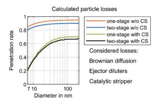
Fig. 2 Calculated particle losses. The losses due to Brownian diffusion are based on calculations according to Hinds<sup>54</sup> with the assumption of a laminar flow inside the tubing. The losses of each ejector diluter were assumed to be 5% according to Giechaskiel et al. 60 The manufacturer of the catalytic stripper determined the respective penetration efficiency at a nominal flow rate of 10 l min<sup>-1</sup>.
