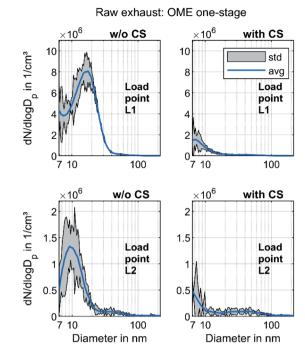
Fig. 5 Particle size distributions of OME raw exhaust with and without volatile particle remover and one-stage dilution: filtered average (arithmetic mean) of three recordings and indication of the standard deviation
