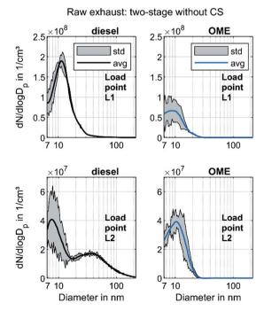
Fig. 3 Particle size distribution of OME and diesel raw exhaust without volatile particle remover and two-stage dilution: filtered average (arithmetic mean) of three recordings and indication of the standard deviation.
