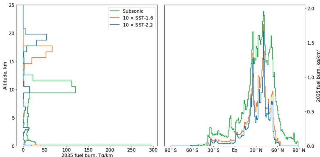
**Fig. 1** Global distribution of aviation fuel burn in 2035 by altitude (left) and latitude (right). The vertical distribution is shown after discretization onto the 72 vertical layers used by the GEOS-Chem model. Values for the supersonic fleets are multiplied by 10 for the sake of clarity.
