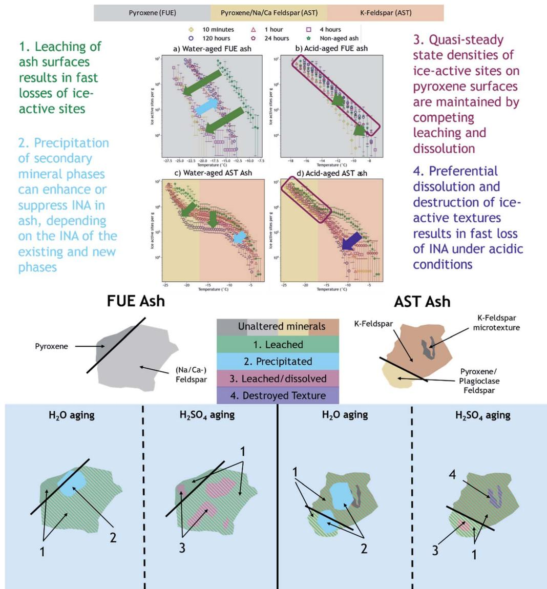
Fig. 4 Attribution of ice nucleation spectral features to specific mineral phases and summary of proposed mechanisms by which chemical aging impacts the INA of FUE and AST ash. Note the full composition of each ash is not represented because not all minerals are expected to contribute to the observed ash INA.
