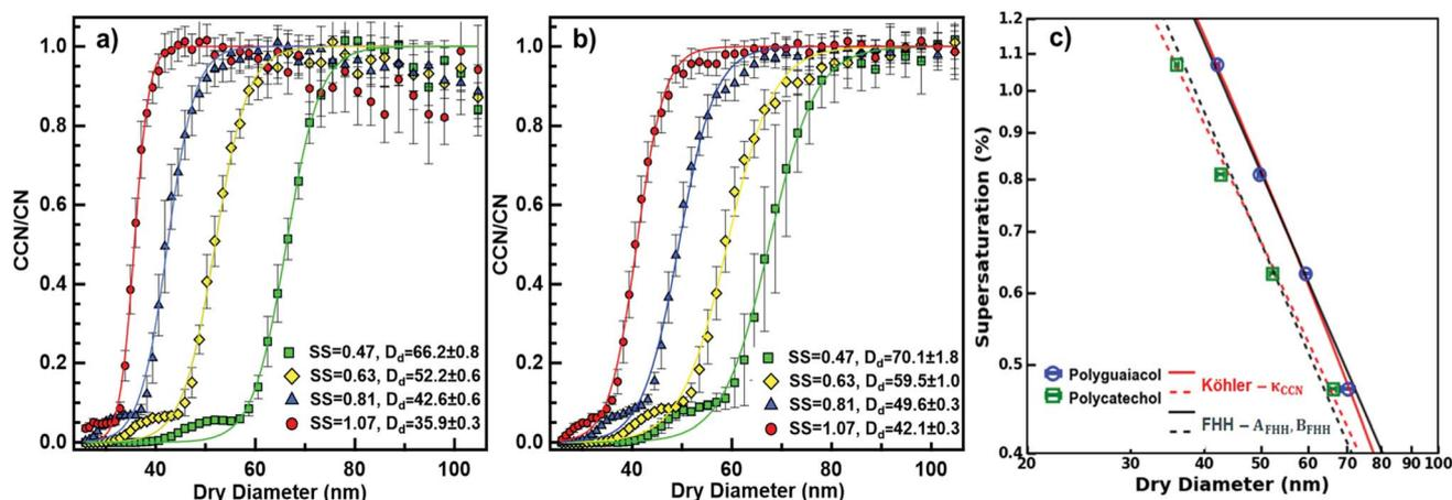
Fig. 2 CCN measurements and analysis. CCN/CN activation *versus* particle dry diameter for (a) polycatechol and (b) polyguaiacol at 4 different supersaturations. Each sigmoid fit (solid line) is the best fit average of 10 measurements. Error bars are standard deviation. (c) Köhler theory (red lines) and FHH model-based power law fits (black lines) of the CCN activity measurements of polycatechol and polyguaiacol. The derived FHH parameters can also be applied to subsaturated measurements.
