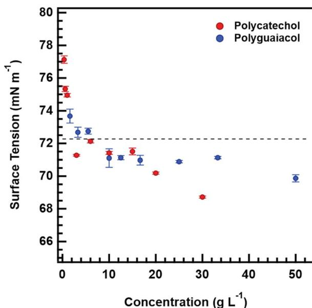
Fig. 5 Surface tension measurements for polycatechol (red circles) and polyguaiacol (blue circles). Horizontal line represents pure water, ST = 72.27 mN m<sup>-1</sup>. Room temperature: 21.8 °C. Error bars represent standard deviation.
