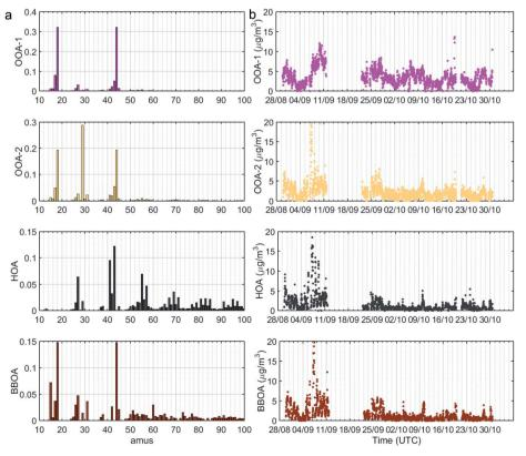
Results from the PMF analyses of ACSM OA data. (a) PMF factor mass spectra profiles and (b) PMF factor mass loading time series.
