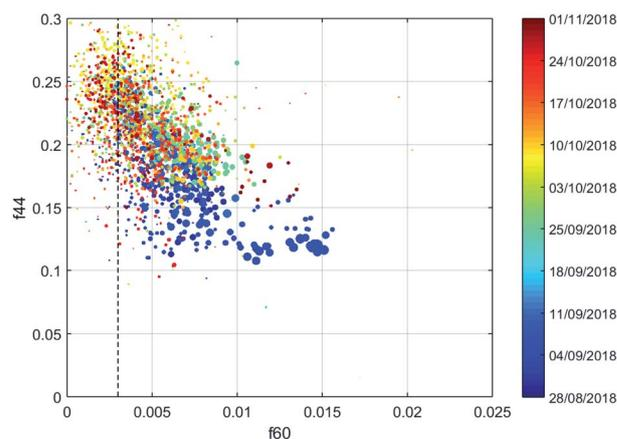
**Fig. 4** Mass fractions  $f_{44}$  vs.  $f_{60}$  in the mass spectra of ambient OAs colored by time and dot size proportional to  $\text{PM}_{10}$  mass loading. The dashed line represents a considered threshold for negligible influence by biomass burning ( $f_{60} = 0.003$ ).
