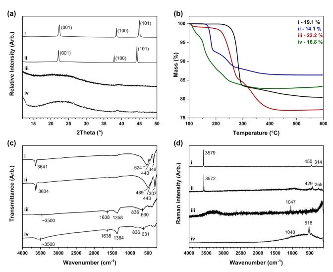
Fig. 2 Data collected of (i)  $\beta$ -Ni(OH)<sub>2</sub>, (ii)  $\beta$ -Co(OH)<sub>2</sub>, (iii)  $\alpha$ -Ni(OH)<sub>2</sub> and (iv)  $\alpha$ -Co(OH)<sub>2</sub>. (a) Powder X-ray diffraction patterns collected with Co K<sub> $\alpha$ 1</sub> radiation ( $\lambda$  = 1.7889 Å), (b) thermogravimetric analysis weight loss data with decomposition to NiO and Co<sub>3</sub>O<sub>4</sub>, (c) infrared absorption spectra as Csl disks and (d) Raman spectra.
