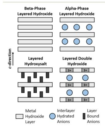
**Fig. 1** Diagram of the structural differences between layered hydroxide phases, layered hydroxysalts and layered double hydroxides showing the variations in anion incorporation.
