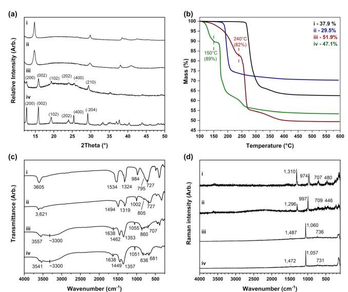
Fig. 3 Data collected of (i)  $Ni_3(OH)_4(NO_3)_2$ , (ii)  $Co_3(OH)_4(NO_3)_2$ , (iii)  $Ni_3(OH)(NO_3) \cdot H_2O$  and (iv)  $Co_3(OH)(NO_3) \cdot H_2O$ . (a) Powder X-ray diffraction patterns collected with Co  $K_{\alpha 1}$  radiation ( $\lambda = 1.7889$  Å), (b) thermogravimetric analysis weight loss data with decomposition to NiO and  $Co_3O_4$ , (c) infrared absorption spectra as CsI disks and (d) Raman spectra.
