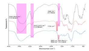
Fig. 1 FTIR spectrum of pristine cellulose nanocrystals derived from cotton by sulfuric acid hydrolysis (black), chlorinated CNCs from SOCl<sub>2</sub> in DMF (red) and TAEA-modified cellulose (blue).
