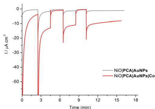
**Fig. 4** Chopped-light chronoamperometric measurements of NiO|PCA| $\beta$ -CD-AuNPs and NiO|PCA| $\beta$ -CD-AuNPs|Co photocathodes at an applied bias of  $-0.1 \text{ V vs. Ag/AgCl}$  in pH 5 MES buffer.
