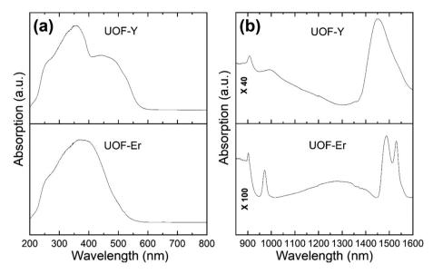
Fig. 4 The DRS spectra of UOF-Er and UOF-Y in the (a) UV-vis and (b) the near infrared regions.
