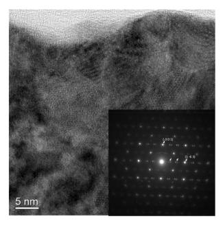
Fig. 3 HRTEM of UOF-Er: a high-resolution TEM image with an inset of a selected area electron diffraction pattern viewed down the [3 5 9] zone axis, also highlighting Bragg maxima from a modulated structure (arrows) along the  $(1-6\ 3)$  direction indicating a  $3\times$  superstructure.
