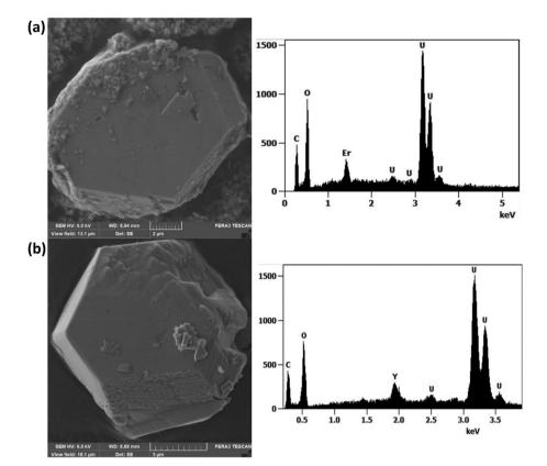
Fig. 1 SEM analysis of (a) UOF-Er and (b) UOF-Y: secondary SEM images of the crystals on the left and their corresponding EDS spectra on the right confirming the presence of both U and the Er/Y in a ~5.5:1 atomic ratio.
