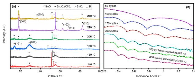
**Fig. 6** (a) GIXRD patterns of the as-deposited films including reflections of SnO, Si, SnO<sub>2</sub>, and Sn<sub>3</sub>O<sub>2</sub>(OH)<sub>2</sub> and (b) XRR patterns of the films grown at different deposition temperatures and cycles, as well as annealed films (the black dashed lines in the XRR graph are simulated patterns).
