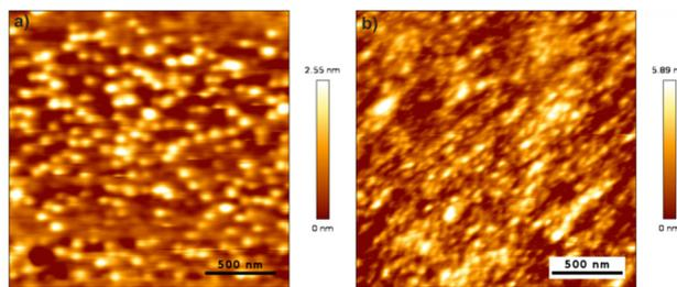
**Fig. 7** AFM image of a 2 × 2 μm<sup>2</sup> area of SnO deposited on Si(100) at 220 °C. Film thicknesses are (a) 7 nm and (b) 18 nm.
