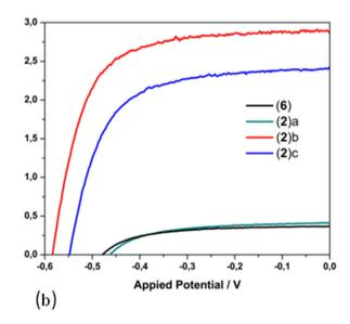
Fig. 13 J-V curves for the copper(i)-based dyes 1,  $[Cu(pqcame_2)][PF_6]$  (A) (a); 2 and 6 (b). Lower case letters highlight the different architecture of the semiconductor material of the anode, dyed with 1 and 2, as reported in Table 2.
