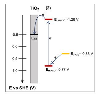
Fig. 12 The energy diagram of the photoelectrode electrolyte interface depicting the HOMO-LUMO energy levels of dye (2) vs. the conduction band (CB) level of  $TiO_2$  and the redox potential of  $I^-/I_3^-$ .
