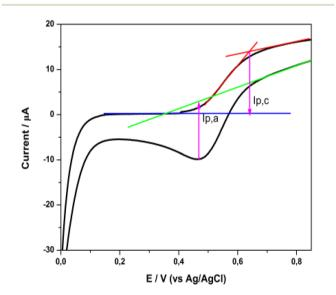
Fig. 11 Cyclic voltammogram of a 2 sensitized titania film, in a three-electrode electrochemical cell.
