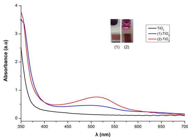
Fig. 10 Dyes 1 and 2 adsorbed on TiO<sub>2</sub>.
