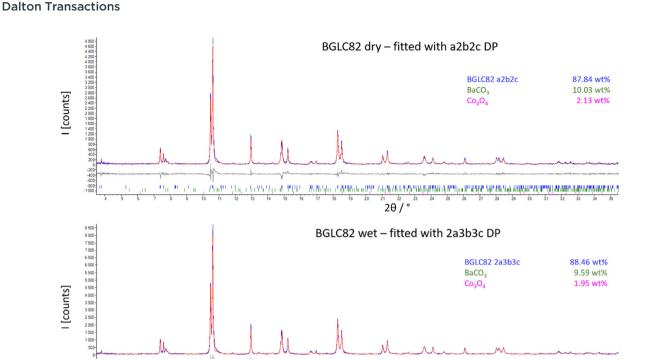
Fig. 8 SR-PXD of BGLC82 treated in dry (upper) and wet (lower) atmosphere at 300 °C. The spectra are fitted to a *Pmmm* a2b2c (dry), and a *Pmmm* 2a3b3c (wet) unit cell.
