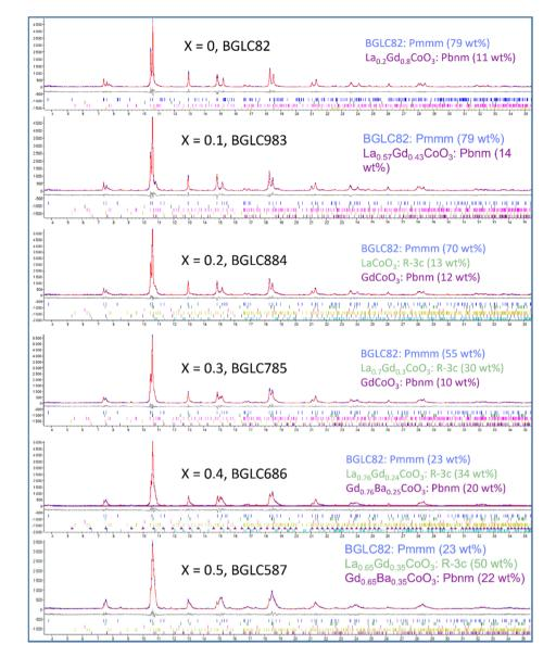
Fig. 2 SR-PXD rietveld refinements (red line) of BGLC (x = 0-0.5, y = 0.2). Minority phases  $Co_3O_4$ ,  $Gd_2O_3$  and  $BaCO_3$  are refined, but omitted in the figure legends.
