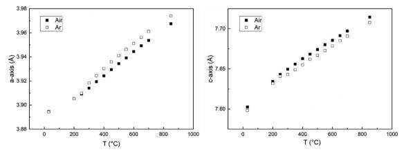
Fig. 13 Cell parameters for a-axis (left) and c-axis (right) vs. temperature for x = 0.1 in air (closed squares) and Ar (open squares) atmospheres.
