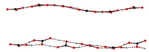
Fig. 2 Bicarbonate chains in the crystal structure of 4, sinusoidal (top) and twisted (bottom).
