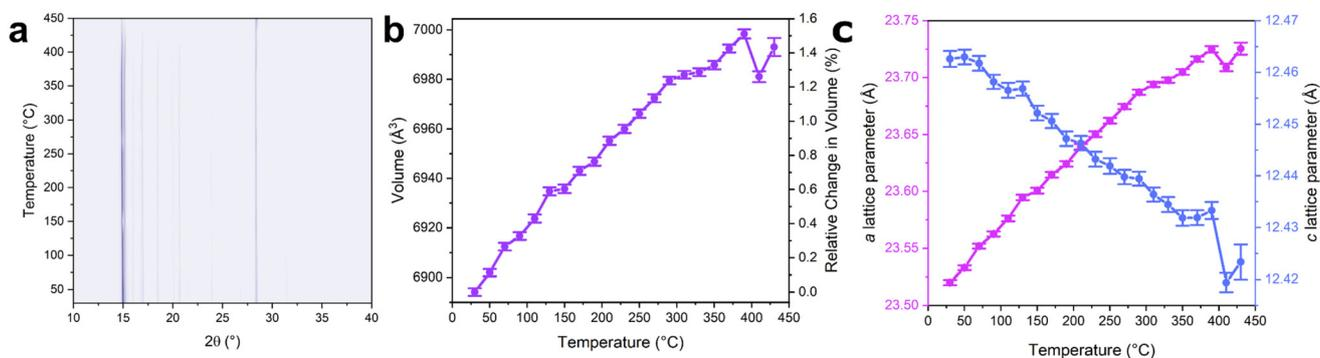
**Fig. 3** Contour plot of diffraction data as a function of temperature for ZIF-zni (a). The high intensity reflection at *ca.* 28.5° 2θ is from the silicon standard. Change in unit cell volume (b) and lattice parameters (c) as a function of temperature. Volume parameters were extracted from Rietveld refinements of the diffraction data (Fig. S14–S17, Tables S2–S4†).
