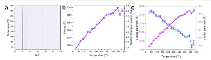
Fig. 3 Contour plot of diffraction data as a function of temperature for ZIF-zni (a). The high intensity reflection at ca. 28.5°  $2\theta$  is from the silicon standard. Change in unit cell volume (b) and lattice parameters (c) as a function of temperature. Volume parameters were extracted from Rietveld refinements of the diffraction data (Fig. S14-S17, Tables S2-S4†).
