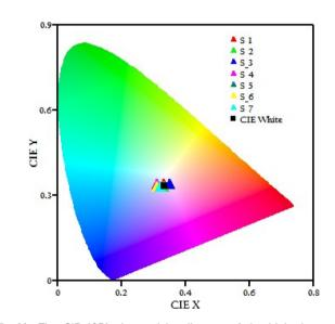
Fig. 11 The CIE 1931 chromaticity diagram of the biphasic samples with mixing ration referred at Table 1 with excitation of 980 nm lasers.
