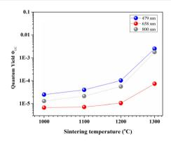
Fig. 7 Sample sintering temperature dependence of the absolute quantum yield  $\Phi_{UC}$  of the major and minor emission bands of Tm<sup>3+</sup>/ Yb<sup>3+</sup>:BCZT ceramics.
