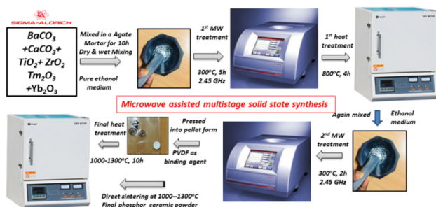
Fig. 1 Modified MW assisted multistage solid state synthesis flowchart of BCZT:Tm 3+ /Yb 3+ ceramic phosphor.
