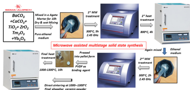
Fig. 1 Modified MW assisted multistage solid state synthesis flowchart of \text{BCZT:Tm}^{3+}/\text{Yb}^{3+} ceramic phosphor.
