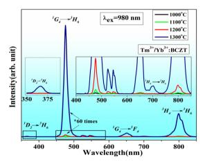
Fig. 4 Upconversion emission spectra with optical transitions of bands for Tm3+/Yb3+:BCZT ceramics at different sintering temperatures, measured at 980 nm diode laser excitations with  $P_{\rm exc}$  = 35 W cm<sup>-2</sup>.
