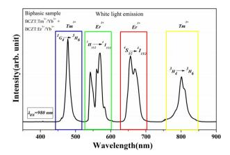
Fig. 9 Typical emission spectra of white emitting biphasic sample (Tm<sup>3+</sup>/Yb<sup>3+</sup>:BCZT + Er<sup>3+</sup>/Yb<sup>3+</sup>:BCZT) under 980 nm excitation.
