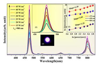
**Fig. 5** Excitation power dependence UC emission spectra of the emission bands of  $Tm^{3+}/Yb^{3+}$ :BCZT ceramics. Inset (1) shows perfect Gaussian distribution of the 479 nm blue-emitting band from the sample. Inset (2) shows double logarithmic plots corresponding power density-dependent slope factors "n". Inset (3) shows intense blue emission from the sample ( $P_{\rm exc} = 35~{\rm W~cm}^{-2}$ ) directly visible through naked eyes, captured using digital mirror less camera.
