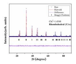
Fig. 3 Structural investigation and Rietveld refinement results for the  $Tm^{3+}/Yb^{3+}$  doped BCZT sample sintered at 1300 °C.
