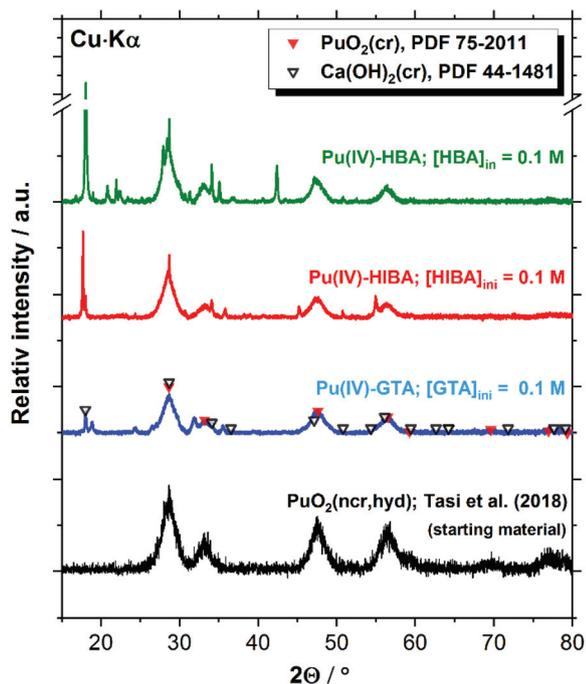
Fig. 10 XRD patterns of the Pu(IV) solid phase used as starting material (as reported in (Tasi *et al.*, 2018)), and the corresponding solid phases after equilibration in the solubility experiments with GTA, HIBA and HBA at  $[L]_{\text{tot}} = 0.1$  M, in all cases containing HQ as redox buffer. Symbols reproduce the patterns reported for  $\text{PuO}_2(\text{cr})$  (PDF-75-2011) and portlandite ( $\text{Ca}(\text{OH})_2(\text{cr})$ , PDF-44-1481) reference materials.
