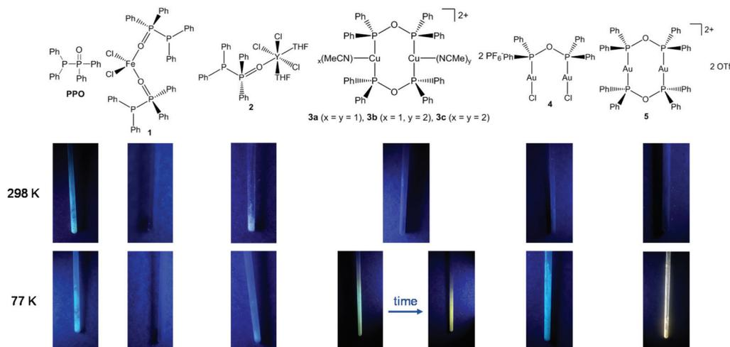
**Fig. 9** Images of the PPO ligand and the complexes **1–5** under UV light radiation (365 nm) at room temperature and under liquid N<sub>2</sub> cooling.
