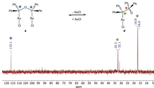
Fig. 3  $^{31}\text{P}\{^1\text{H}\}$  NMR spectrum of complex **4** in  $\text{CDCl}_3$ , indicating the presence of the PPO-containing gold complex **4'**. Note: A small amount of impurities (30.8 ppm) was observed, since **4** is readily hydrolysed.
