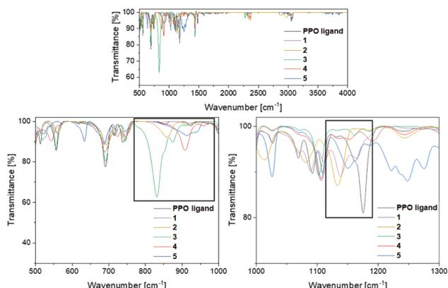
Fig. 4 FT-IR spectra of the PPO ligand and the transition metal complexes **1–5** in the region of  $500\text{--}3250\text{ cm}^{-1}$ . Top: overview spectrum, bottom: of the POP (left) and PPO (right)-relevant regions.
