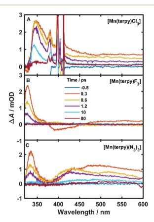
Fig. 2 Difference spectra at various pump-probe time delays of all complexes. (A) [Mn(terpy)Cl<sub>3</sub>] after exciting at 400 nm. The spikes around 400 nm are from pump scatter. (B) [Mn(terpy)F<sub>3</sub>] after exciting at 750 nm. The small signals in the visible region at 0.3 ps are from solvent oscillations. (C) [Mn(terpy)( $N_3$ )<sub>3</sub>] after exciting at 800 nm.
