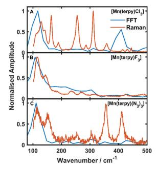
Fig. 4 Fast Fourier transforms of the residuals of the kinetic fit plotted with the low frequency Raman spectra. (A-C) refer to [Mn(terpy)Cl<sub>3</sub>], [Mn(terpy) $F_3$ ] and [Mn(terpy)( $N_3$ ) $_3$ ], respectively. The peak in the FFT at 110 cm<sup>-1</sup> matches well with the frequencies from the kinetic trace fitting. The second peak in the Raman in [Mn(terpy)Cl<sub>3</sub>] occurring at  $400 \text{ cm}^{-1}$  is a response from the solvent (Fig. S8†).
