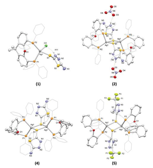
Fig. 1 Views of the molecular structures of 1, 2, 4 and 5 with displacement ellipsoids shown in the 30% probability level. In all cases, selected C atoms are drawn in wireframe for clarity reasons, while H atoms are omitted, except from the H atoms of the NH groups of the thioamide ligands in 1 and 2.
