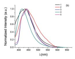
Fig. 2 (a) UV-Vis electronic absorption spectra and (b) emission spectra (excitation at 320 nm) of 1-5 in DMSO solutions ( $\sim 5 \times 10^{-5}$  M).
