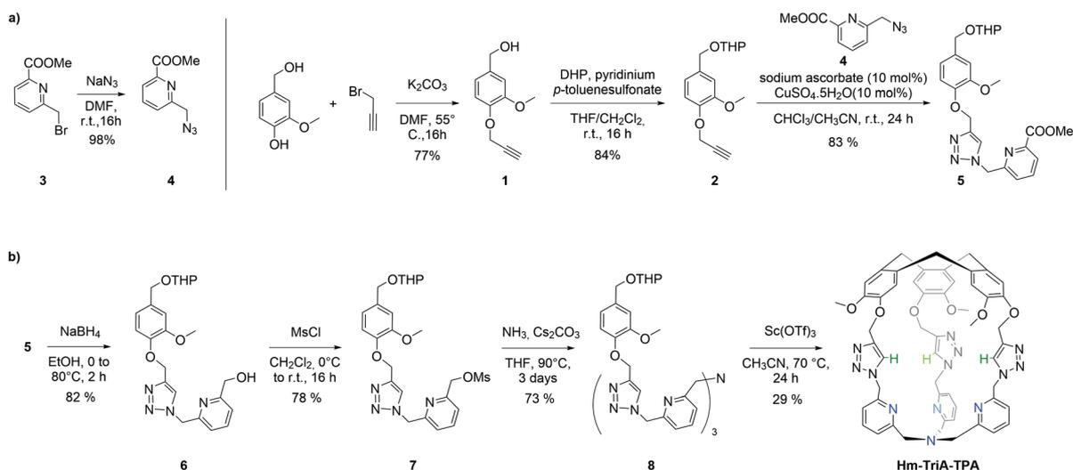
**Scheme 1** (a) Synthesis of the pyridine-triazole precursor 5. (b) Synthesis of the targeted hemicryptophane **Hm-TriA-TPA**.
