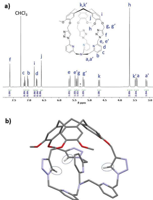
**Fig. 1** (a)  $^1\text{H}$  NMR spectra ( $\text{CDCl}_3$ , 400 MHz) of **Hm-TriA-TPA** along with (b) view of its X-ray crystal structure. Only the hydrogen atoms belonging to the three triazole units have been included for clarity.
