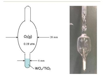
Fig. 1 Diagram and actual picture of a quartz cell used for measuring Raman spectra under static equilibrium. The cell is sealed under  $O_2(g)$ ,  $p_{O_2} = 0.19$  atm.
