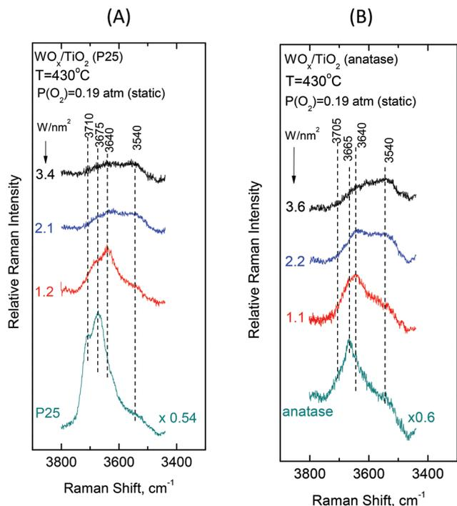
**Fig. 12** Dependence on surface coverage at  $T = 430\text{ °C}$  for (A)  $\text{WO}_x/\text{TiO}_2(\text{P25})$  and (B)  $\text{WO}_x/\text{TiO}_2(\text{anatase})$ . Raman spectra at static equilibrium under  $p_{\text{O}_2} = 0.19\text{ atm}$  for samples with  $W$  surface densities ( $\text{W nm}^{-2}$ ) as indicated by each spectrum. Each panel includes the Raman spectrum of the corresponding pure  $\text{TiO}_2$  support at  $430\text{ °C}$  as reference.
