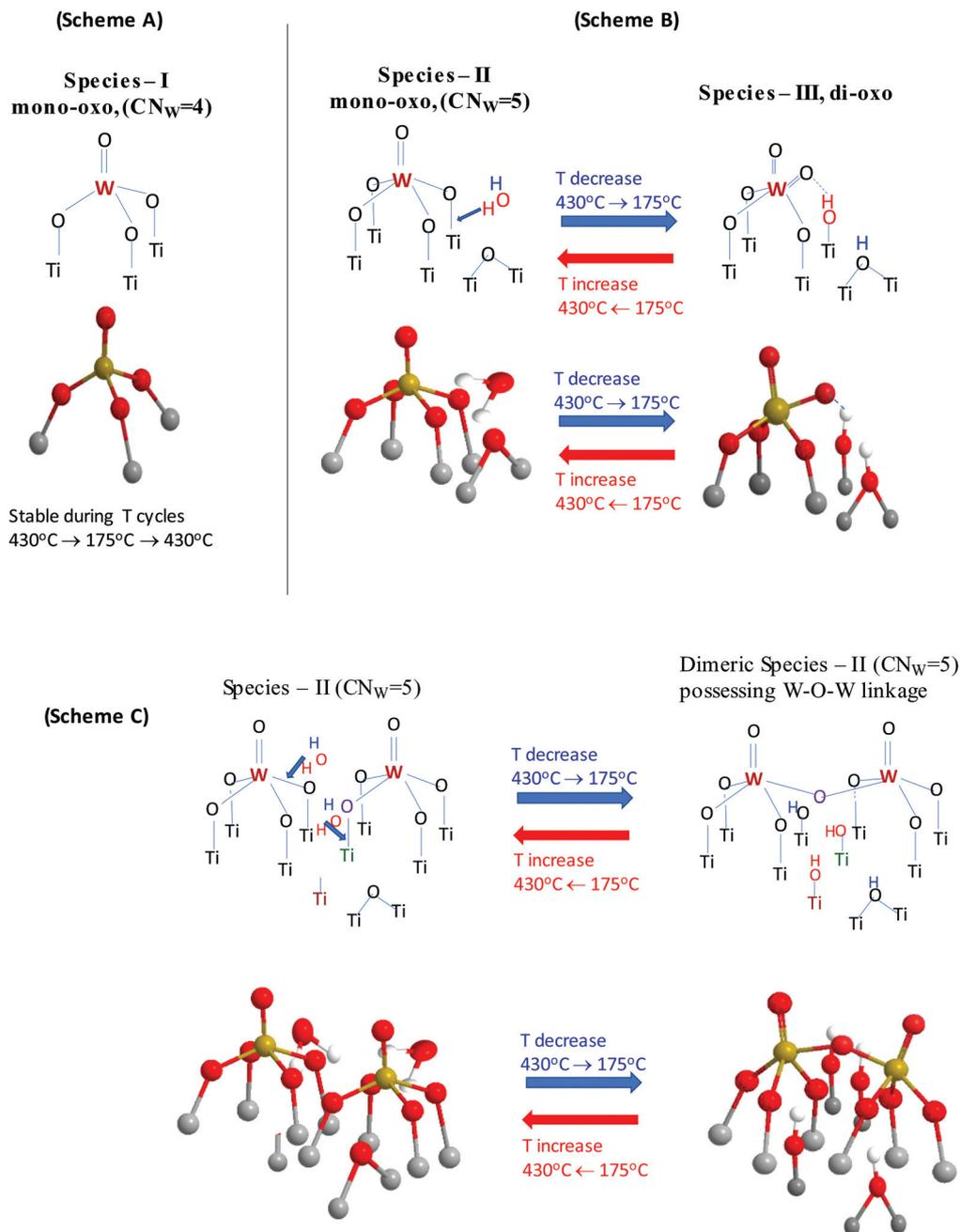
**Fig. 16** Temperature dependent structural transformations. Scheme (A) highlights the stability of Species-I in the 430 °C → 175 °C → 430 °C cycle. Scheme (B): molecular level mechanism of Species-II ↔ Species-III T-dependent transformation. Scheme (C): molecular level mechanism of Species-II association via W–O–W bridging linkages.
