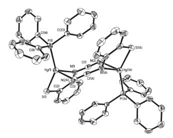
Fig. 2 Molecular structure of  $[Hg{SC_6H_4N(C\equiv N)}(PPh_3)]_2$  4a.<sup>8</sup> Thermal ellipsoids are displayed at 50% probability and hydrogen atoms omitted for clarity. Selected bond lengths (Å) and bond angles (°): Hg1-N1 2.312(4), Hg1-S1 2.352(2), Hg1-P1 2.373(2), Hg1-N2A 2.517(5), N1-C1 1.287(6), N2-C1 1.153(6), S1-Hg1-N1 81.76(11), N1-Hg1-N2A 91.86(14), S1-Hg1-P1 147.76(5), N1-Hg1-P1 122.04(11), N1-C1-N2 176.2(6).
