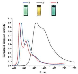
Fig. 7 Normalized emission spectra of chloro-platinum complexes 1–3 in deoxygenated CH<sub>2</sub>Cl<sub>2</sub> solution ( $c \sim 10^{-5}$  M).  $\lambda_{\rm exc} = \lambda_{\rm max}^{\rm abs}$  of the lowest energy band inset: picture of CH<sub>2</sub>Cl<sub>2</sub> solution taken under UV irradiation.
