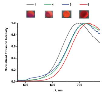
Fig. 9 Normalized emission spectra of complexes 1, and 4–6 in KBr matrix (2 w%).  $\lambda_{\rm exc} = \lambda_{\rm max}^{\rm abs}$  of the lowest energy band in CH<sub>2</sub>Cl<sub>2</sub> solution inset: picture of KBr pellets taken under UV irradiation.
