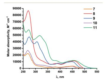
Fig. 6 Absorption spectra of alkynyl-platinum complexes 7–11 in  $CH_2Cl_2$  ( $c\sim 10^{-5}$  M).
