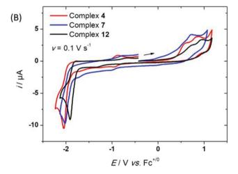
Fig. 4 Cyclic voltammetry (CV) at a Pt working electrode (E/V vs. Fc<sup>+</sup>/Fc) of (A) chloro-platinum complexes **1**, **2** and **3** ( $v = 0.1 \text{ V s}^{-1}$ ) and (B) alkynyl-platinum complexes **4**, **7** and **12** in CH<sub>2</sub>Cl<sub>2</sub>/NBu<sub>4</sub>PF<sub>6</sub> 0.1 M under inert atmosphere. C = 0.5 mM. Inset (A): CV of complex **1** at  $v = 5 \text{ V s}^{-1}$ .
