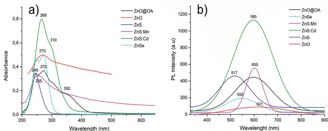
**Fig. 5** Characterization of Qds, (a) UV/Vis spectra; (b) PL spectra of Qds.
