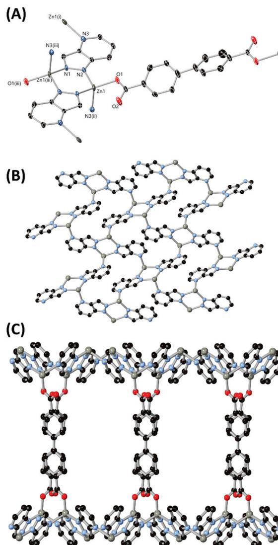
Fig. 2 (A) Metal and ligand environment in the structure of **1**. ADPs are rendered at the 50% probability level and hydrogen atoms are omitted for clarity. (B) The metal–azolate layer in the structure of **1**, carboxylate groups not shown; (C) the **bpdc** linkages between metal–azolate layers in the structure of **1**. Symmetry codes used to generate equivalent atoms: (i)  $+x, 1 - y, z - 1/2$ ; (ii)  $+x, 1 - y, z + 1/2$ ; (iii)  $3/2 - x, 1/2 - y, 1 - z$ .
