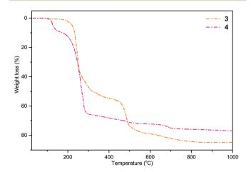
TGA curves for 3 and 4 measured at a heating rate of 10 °C under a nitrogen atmosphere over the temperature range 25-1000 °C.
