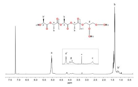
Fig. 12 <sup>1</sup>H NMR spectrum of 3-arm PLLA in C<sub>6</sub>D<sub>6</sub>, \* – assigned ligand residues.
