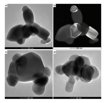
Fig. 9 TEM micrographs of  $\beta\text{-LiGaO}_2$  prepared by calcination of 4 at 850 °C (a–d).
