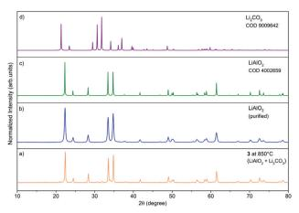
Fig. 6 PXRD patterns of materials prepared by calcination of  $\bf 3$  at 850 °C (a), purified  $\gamma$ -LiAlO<sub>2</sub> (b),  $\gamma$ -LiAlO<sub>2</sub> [Crystallography Open Database (COD), 4002659, green] (c), Li<sub>2</sub>CO<sub>3</sub> [COD, 9009642, purple] (d).
