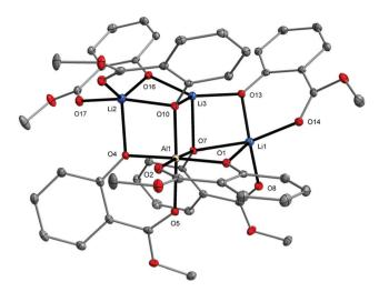
Fig. 3 Molecular structure of [AlLi<sub>3</sub>(MesalO)<sub>6</sub>] (3). The displacement ellipsoids are drawn at the 30% probability level. Hydrogen atoms are omitted for the sake of clarity.
