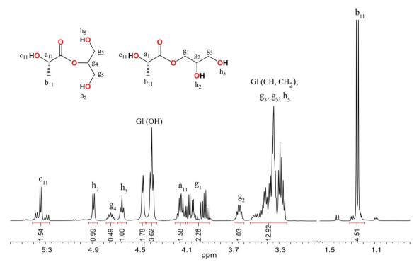
Fig. 10  $^{1}$ H NMR spectrum in DMSO-D<sub>6</sub> of GlL<sub>1</sub> synthesized in the L-LA alcoholysis reaction in the presence of 3.
