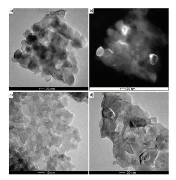
Fig. 8 TEM micrographs of  $\gamma$ -LiAlO $_2$  prepared by calcination of 3 at 850 °C (a-d).
