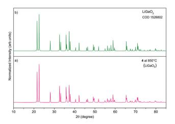
Fig. 7 PXRD patterns of the material prepared by calcination of 4 at 850 °C (a),  $\beta$ -LiGaO<sub>2</sub> [COD, 1526802, green] (b).
