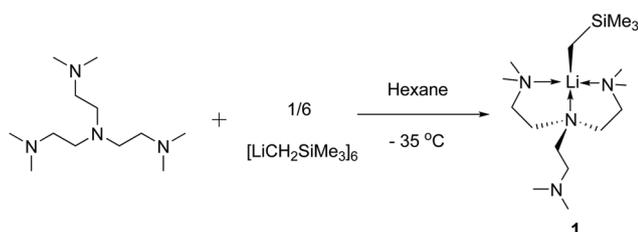
**Scheme 2** Synthesis of the  $\text{LiCH}_2\text{SiMe}_3$  monomer  $[\text{Li}(\text{CH}_2\text{SiMe}_3)(\kappa^3\text{-}N,N',N''\text{-Me}^6\text{Tren})]$  (**1**).
