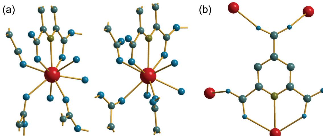
**Fig. 3** (a) The local environment of the two Ce sites in (2) with cut-off bonds showing connection to neighbouring atoms. (b) The connectivity of one of the PTC ligands in (2); the second PTC ligand has identical connectivity and is not shown. In both cases, red spheres are cerium, grey are carbon, blue are oxygen, olive are nitrogen and hydrogens are not shown.
