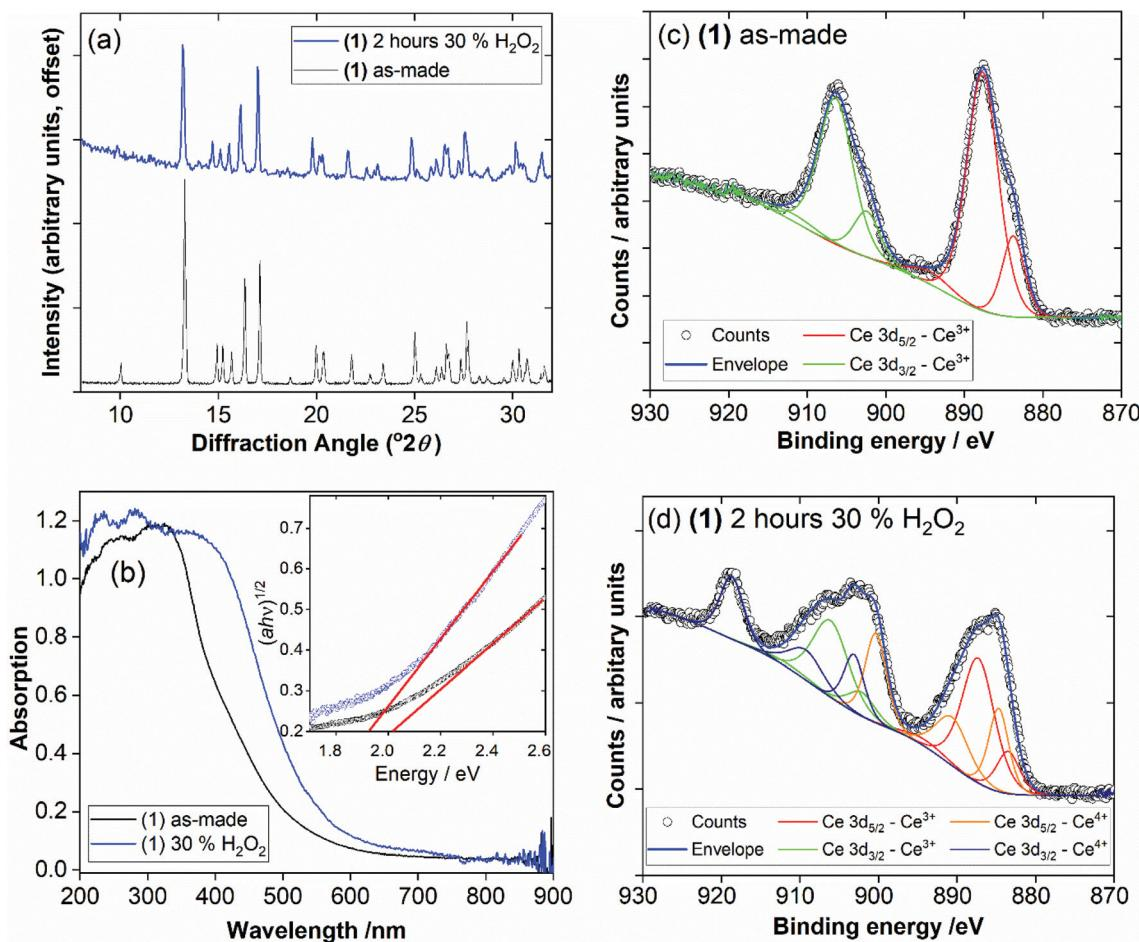
**Fig. 9** Characterisation of (1) upon application of oxidising conditions: (a) powder XRD measured before and after exposure to 30%  $\text{H}_2\text{O}_2$  solution, (b) UV-Vis of the two solids, with Tauc plots inset, where red lines showing the linear extrapolation to estimate band gap, and (c) and (d) XPS of the materials, with the deconvolution and assignment of signals indicated.
