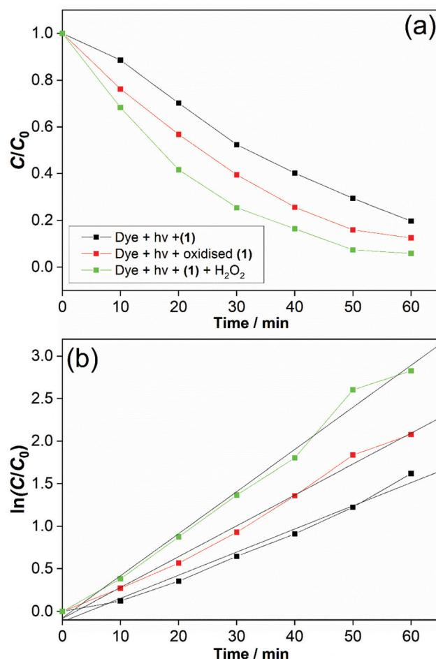
**Fig. 10** (a) Photodegradation of methyl orange at catalysts, 25 °C, UV light (250 W). (b) Kinetic fit of the time trace and linear plots (pseudo first-order) of the UV-VIS band at  $\lambda_{\text{max}} = 505$  nm,  $R^2 = 0.982$  (black line), 0.992 (red line) and 0.987 (green line). The legend in (b) is the same as in (a).
