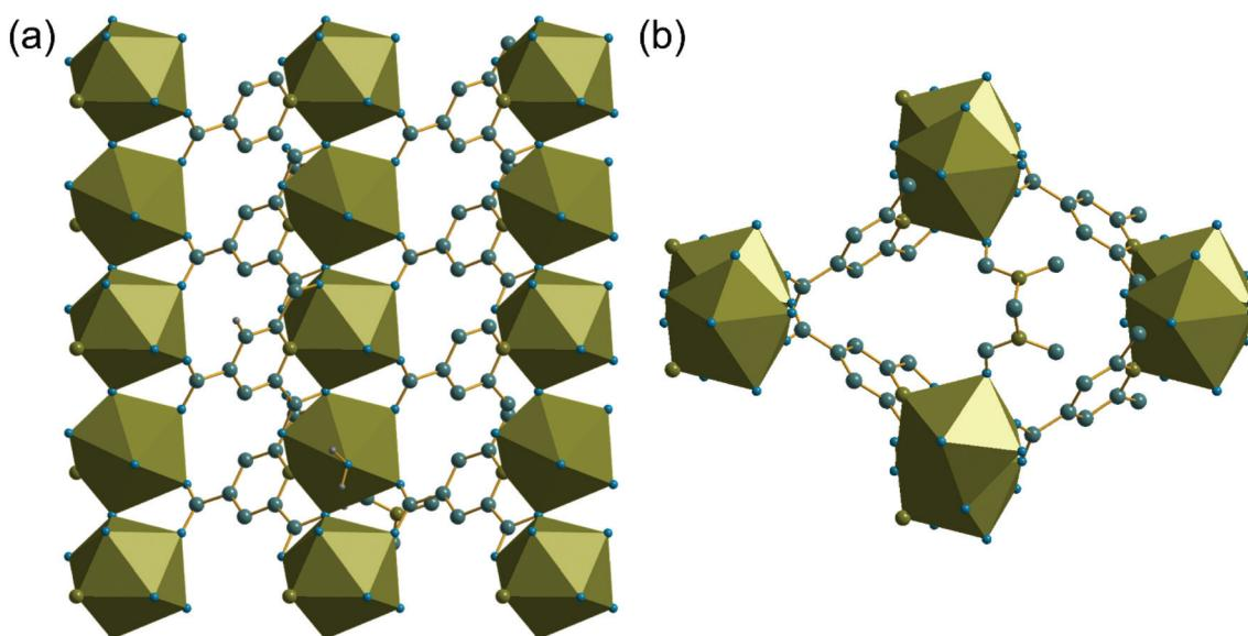
Fig. 7 (a) View of (3) along *b* showing cross-linked chains of corner-shared cerium-centred polyhedra. (b) Projection of (3) along *c* showing co-ordinated DMF (one orientation shown) filling extra-framework space. The cerium environment is represented by the polyhedra, and grey spheres are carbon, blue are oxygen, olive are nitrogen and hydrogens are not shown.
