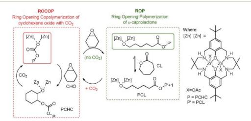
Fig. 9 Williams and coworkers switchable dizinc catalyst for ROP and ROCOP. Copyright (2014) Wiley. Used with permission from ref. 104.
