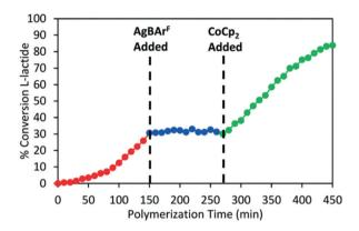
Fig. 3 Time vs. conversion plot of redox switchable ROP of L-LA using Zr complex 8b<sup>red/ox.50</sup> The oxidised species 8b<sup>ox</sup> was generated in situ by addition of AgBAr<sup>F</sup> (blue circles) and the reduced species was regenerated by CoCp2 (green circles). Reproduced from ref. 50 with permission from the Royal Society of Chemistry.
