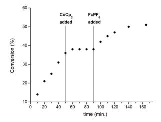
Fig. 1 A plot of conversion vs. time for the polymerisation of CHO using  $7^{\text{red/ox}}$  (2 mol%). [Copyright (2016) Wiley. Used with permission from ref. 44].
