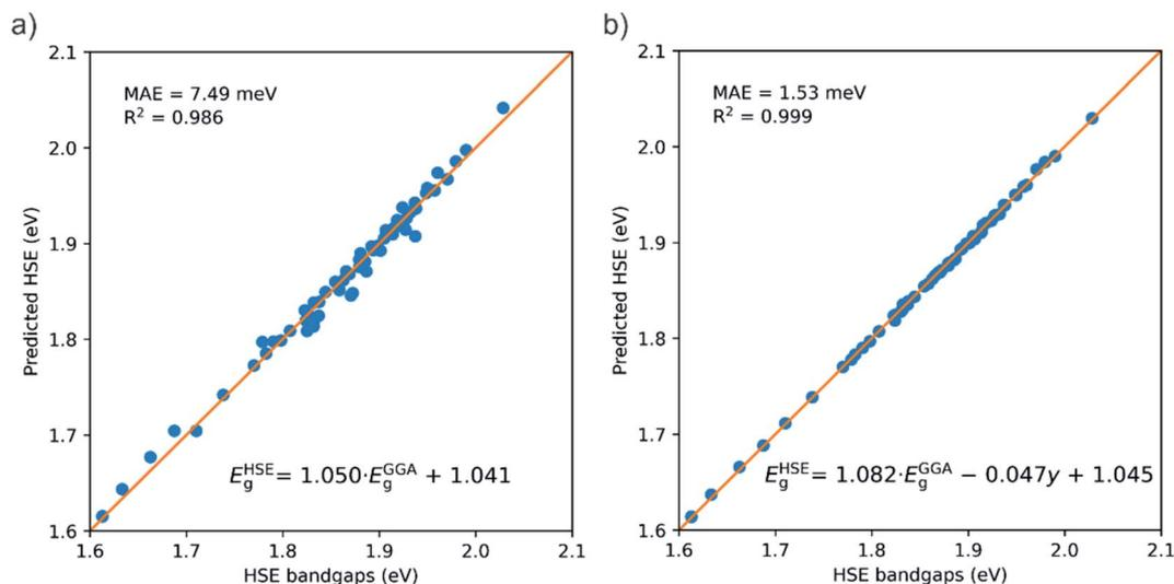
Fig. 2 Performance of two models to predict the HSE bandgaps from the GGA + U bandgaps: (a) simple linear model not using the inversion degree; and (b) bi-linear model using the inversion degree  $\gamma$  as additional parameter.
