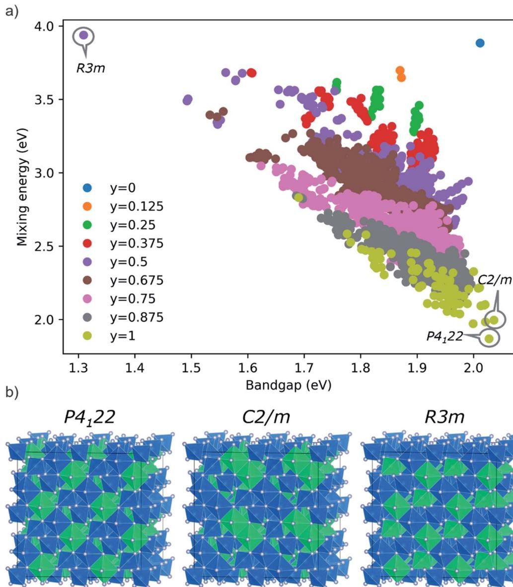
Fig. 8 (a) Distribution of predicted mixing energies and bandgaps for all the inequivalent Ge/Sn configurations in the  $\text{GeSn}_2\text{N}_4$  cubic unit cell. Different colors represent different inversion degrees. (b) Structures of extremal configurations: the  $P4_122$  configuration has the lowest energy, the  $C2/m$  configuration has the widest bandgap, and the  $R3m$  configuration has the narrowest bandgap but highest energy. Sn in blue, Ge in green.
