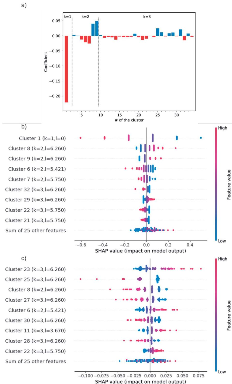
Fig. 6 (a) Linear coefficients for every cluster (for orders  $k = 1, 2$ , and  $3$ ) in the LR model used to predict mixing energies. SHAP analysis of the impact of the different clusters within the CCFs on the predicted values of (b) mixing energy (LR model) and (c) bandgap (MLP model), where  $l$  (in Å) is the maximum distance between atoms of the cluster.
