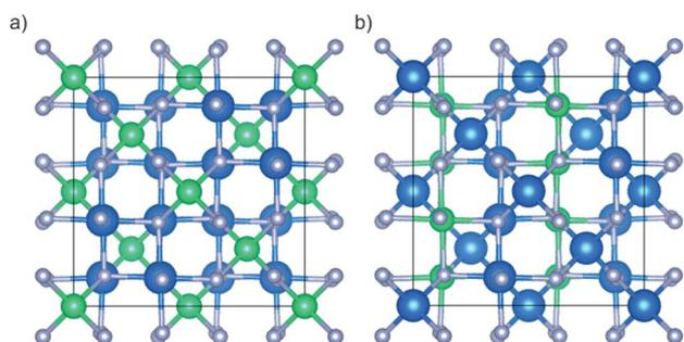
Fig. 1 Structures of the direct ( $y = 0$ ) and an inverse ( $y = 1$ ) GeSn<sub>2</sub>N<sub>4</sub> spinel. Ge: green; Sn: blue; N: gray.
