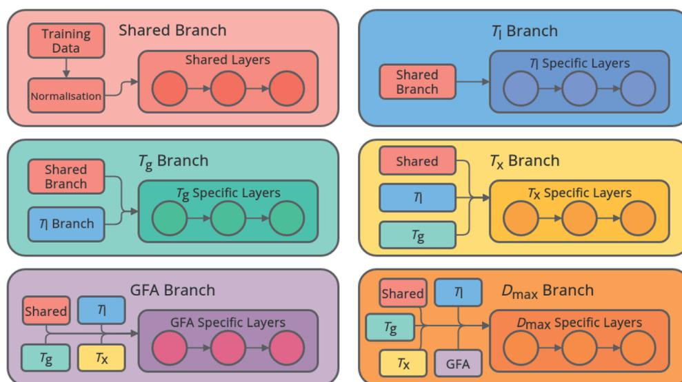
Fig. 1 Architecture of the neural-network models, showing globally accessed shared branches, and sequentially assembled prediction branches for the liquidus temperature,  $T_l$ , the glass-transition temperature,  $T_g$ , the temperature of crystallization onset,  $T_x$ , glass-forming ability (GFA) classification as crystal, glassy ribbon, or bulk metallic glass, and the maximum castable diameter of a fully glassy rod,  $D_{\max}$ .
