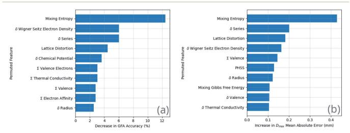
Fig. 9 The top ten most important features as determined by feature permutation applied to the ensemble neural-network model for (a) GFA classification and (b) prediction of the maximum castable diameter of a fully glassy rod, D<sub>max</sub>. The most important features cause the largest decrease in model performance when permutation destroys their relation to the other data.
