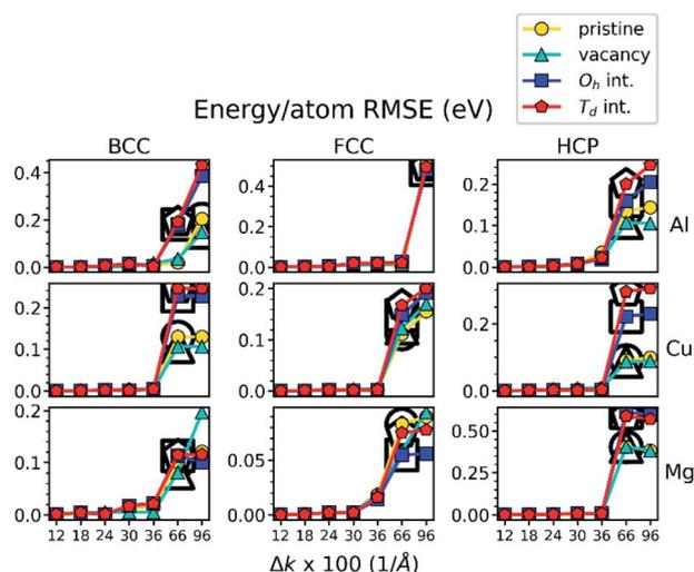
Fig. 4 The E-RMSE of single-point DFT calculations as a function of  $\Delta k$  for the 3600 configurations of the test dataset. Threshold  $\Delta k$  ( $\Delta k_T$ ) determined by the  $\frac{1}{2}$  MAD criterion is highlighted by prominent black-outlined symbols.
