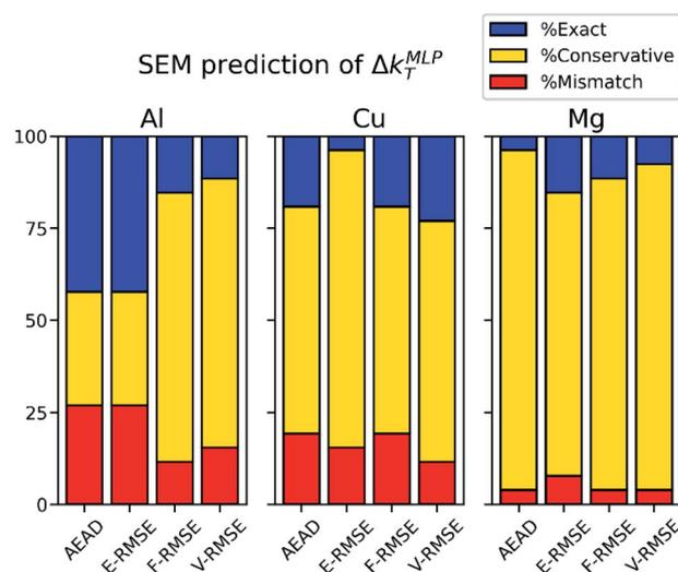
Fig. 5 Analysis of SEM predictions of  $\Delta k_T$  of MLP material properties ( $\Delta k_T^{\text{MLP}}$ ). Proportions of % exact ( $\Delta k_T^{\text{MLP}} = \Delta k_T^{\text{SEM}}$ ), % conservative ( $\Delta k_T^{\text{MLP}} > \Delta k_T^{\text{SEM}}$ ), and % mismatch ( $\Delta k_T^{\text{MLP}} < \Delta k_T^{\text{SEM}}$ ) over all properties, lattices, and structures is indicated for each SEM by blue, yellow, and red shading, respectively.
