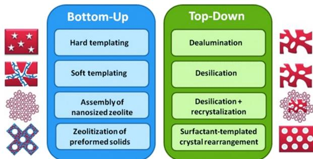
Fig. 2 “Bottom-up” and “top-down” approaches to mesoporous zeolites. Reprinted from ref. 65. Copyright (2013) with permission from John Wiley and Sons.
