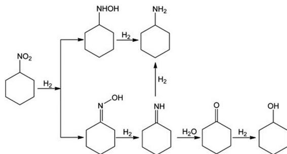
**Scheme 2** Nitrocyclohexane hydrogenation mechanism proposed by Liu *et al.*<sup>53</sup> Reprinted (adapted) with permission from Liu *et al.*<sup>53</sup> Copyright {2013} John Wiley & Sons.
