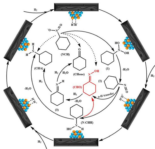
**Scheme 4** Mechanism involving the formation of cyclohexanone oxime over the Cu–Ni/AC catalyst. Reprinted (adapted) with permission from Yao *et al.*<sup>52</sup> Copyright {2021} American Chemical Society.
