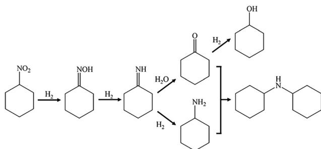
**Scheme 1** Mechanism of nitrocyclohexane hydrogenation proposed by Wang *et al.*<sup>19</sup> Reprinted (adapted) with permission from Wang *et al.*<sup>19</sup> Copyright (2013) Elsevier.
