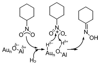
**Scheme 3** Nitrocyclohexane hydrogenation on the acid–base pair site on Au catalysts. Reprinted (adapted) with permission from Shimizu *et al.*<sup>48</sup> Copyright {2011} Elsevier.
